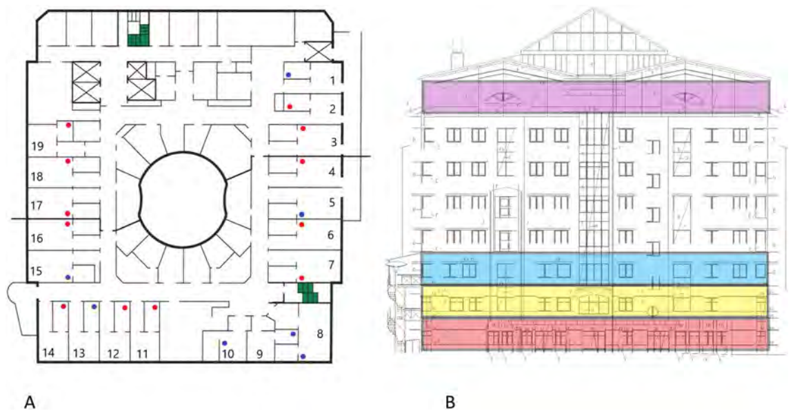
Figure 1. (A) Overview of the 19 investigated COVID-19 ward rooms (ward 1). Dots indicate approximate placing of ceiling vent openings. Red dots indicate openings that where SARS-CoV-2 RNA was detected in at least one of two samplings, blue dots openings negative in both samplings. (B) Lateral view of the hospital building. Ward levels: red; COVID-19 outpatient clinic, yellow and blue; COVID-19 wards 1 and 2, with 19 rooms each, purple; eighth floor with central ventilation fans and HEPA filters. Individual ceiling vent openings were investigated on the second-floor ward (yellow) seen in (A).
